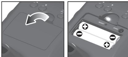
**NOTE** Install batteries in the remote sensor before the main unit. Press **RESET** after each battery change. Do not use rechargeable batteries. We recommend that you use alkaline batteries with this product for longer usage and lithium batteries in temperatures below freezing.
