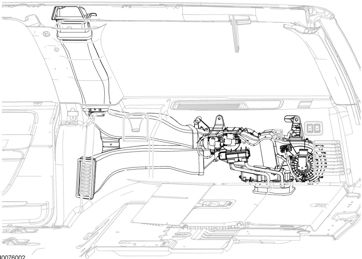
The auxiliary heater core and evaporator core housing is located behind the passenger side lower quarter trim panel. Do not mount any equipment to the housing. Do not mount any equipment in a way that may block the air intake or vents.
