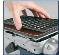
After fitting the sandpaper to the sander align the base of the sander with the hole punch and push down on the sander until the hole punch pierces the sandpaper.
