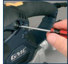
2. Use a small flat screwdriver to unscrew the brush cap and remove the carbon brush assembly.
