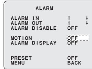
Use the joystick lever (↑↓) to select [MOTION] and use the lever (←→) to select the motion sensor used for alarm detection.
