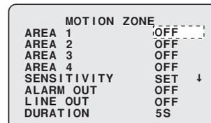
**2** Use the joystick lever (↑↓) to select [AREA (1 - 4)], use the lever (←→) to select "ON ↓", and press the [ENTER] button.
