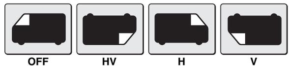
**Memo:** The "HV" option can be used when the camera is installed on the floor. In this option, the direction to which the joystick lever is moved matches the direction to which the camera pans and tilts.
