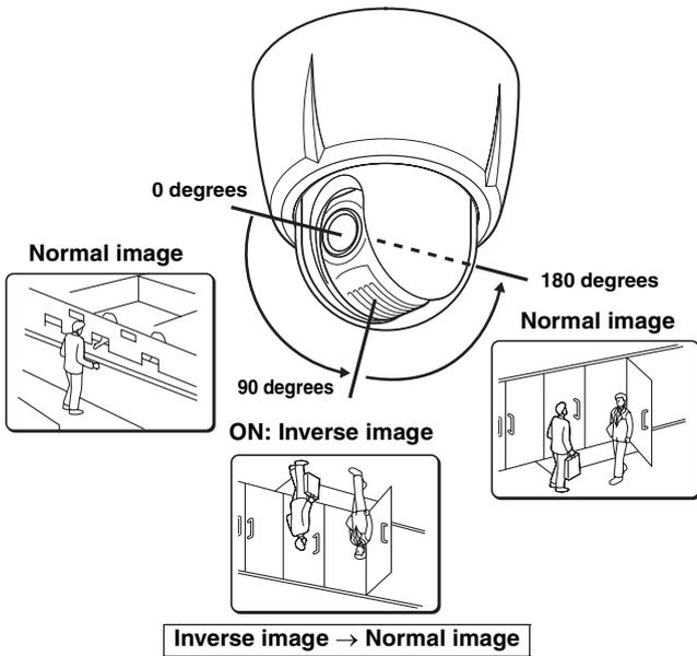
The image is rotated automatically to change inverse image to normal image.
