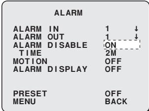
**Memo:** You can also turn on or off the ALARM DISABLE function by using the system controller. Press the [AUX ON] or [AUX OFF] button, and select "8" in the number entry screen.
