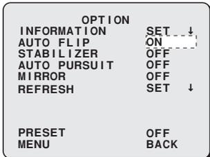
**1** Use the joystick lever (↑↓) to select [AUTO FLIP] and use the lever (←→) to select "ON".
