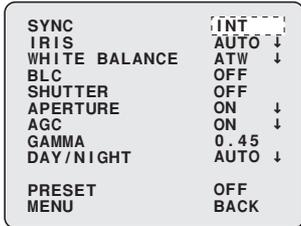
The internal synchronization (INT) is used as an initial setting. In this setting, the vertical synchronization tends to be unstable when multiple cameras are connected through the camera switcher and the camera to be monitored is switched. In this case, use the following steps to adjust the vertical synchronization phase.
