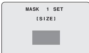
**Memo:** While the lens reaches the tilt end (TILT LIMIT to "OFF"), pressing the [ENTER] button fixes the surveillance image. Use the joystick lever to move the mask pattern to determine the masking position, and press the [ENTER] button.
