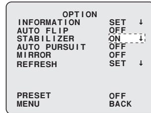
**1** Use the joystick lever (↑↓) to select [STABILIZER] and use the lever (←→) to select "ON ↓", and press the [ENTER] button.
