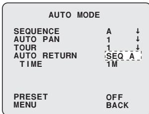
**Memo:** When the AUTO RETURN function has already been enabled, you can turn on or off the function by using the system controller. Press the [AUX ON] or [AUX OFF] button, and select "4" in the number entry screen.
