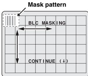
**2** Use the joystick lever (↑↓ or ←→) to move a mask pattern to the area to be excluded in metering, and press the [ENTER] button.
