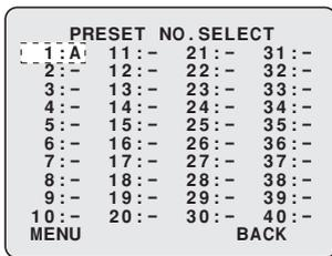
To select a preset number to register the camera's orientation:
