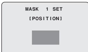
**3** Use the joystick lever to move the surveillance image to determine the masking position, and press the [ENTER] button.
