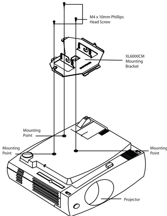
1. Invert the projector and place it on a soft and flat surface. Remove any foot levelers that might possibly prevent the correct installation of the bracket.
