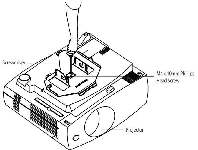
1. Using a screwdriver, secure the XL6000CM mounting bracket using three (3) M4 x 10mm Phillips Head screws. Do not over tighten these screws. Overtightening the screws may result in damaging the threaded inserts on the projector.
