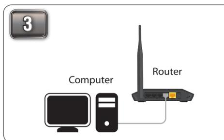
If you are currently using a router, disconnect all the cables connected to it before installing the DIR-605L. Unplug the Ethernet cable from your modem that is connected to your computer. Plug it into the LAN port labeled 1 on the back of your router. The router is now connected to your computer.
