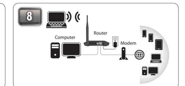
This is a sample network configuration of the setup after you have completed all the setup steps.
