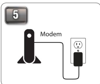
Reconnect the power adapter to your cable or DSL broadband modem and wait for two minutes.
