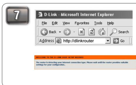
From the computer you connected the router to, open a web browser and enter <http://192.168.0.1> or <http://dlinkrouter>. Press **Enter** and you will be directed to the D-Link Setup Wizard page, which will detect your Internet connection type. Follow the on-screen instructions to configure your Internet settings. After setting up your router, you will be given the option to create a mydlink account. Go to [www.mydlink.com](http://www.mydlink.com) and enter your account information.
