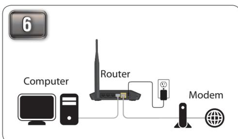
Plug the power back into the modem and power it on. Then connect the supplied power adapter into the power receptor on the back of the router and then plug into a power outlet or surge protector. Verify the power light is lit.
