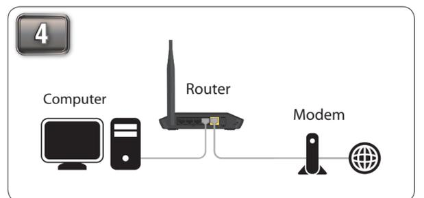
Plug one end of the included blue Ethernet cable that came with your router into the yellow port labeled **INTERNET** on the back of the router. Plug the other end of this cable into the Ethernet port on your modem.
