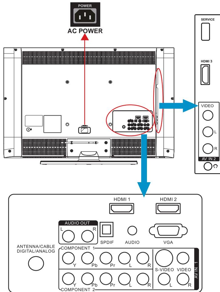
1. **HDMI** – Connect the primary source for digital video such as a DVD multimedia player or set top box through this all digital connector. The white color band on the rear of the TV indicates this connection.
