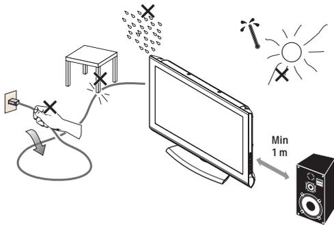
Ensure that the TV is placed in a position to allow free flow of air. Do not cover the ventilation openings on the back cover. To prevent any unsafe situations, no naked flame sources, such as lighted candles, should be placed on or in the vicinity. Avoid heat, direct sunlight and exposure to rain or water. The equipment shall not be exposed to dripping or splashing.
