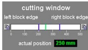
Indication of the left and right block edge, graphically displayed by blue lines. They indicate the maximum horizontal stroke of the microtome sledge on a scale from 0 - 500 mm.
