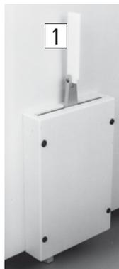
Never leave the instrument unattended when the knee lever is folded out (1) to prevent the microtome from being set in motion accidentally.
