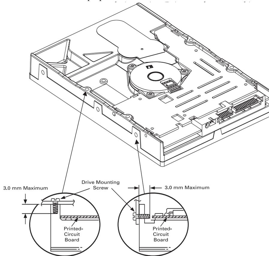
**Figure 4-5** Mounting Screw Clearance
