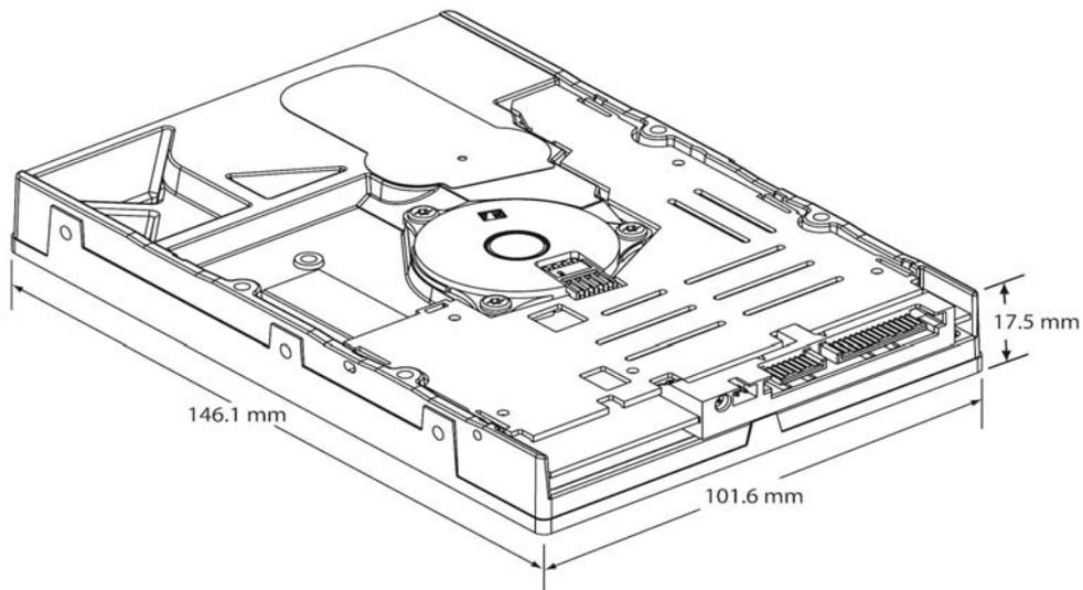
**Figure 4-1** Mechanical Dimensions of Maxtor DiamondMax 8S 40GB SATA Hard Disk Drive
