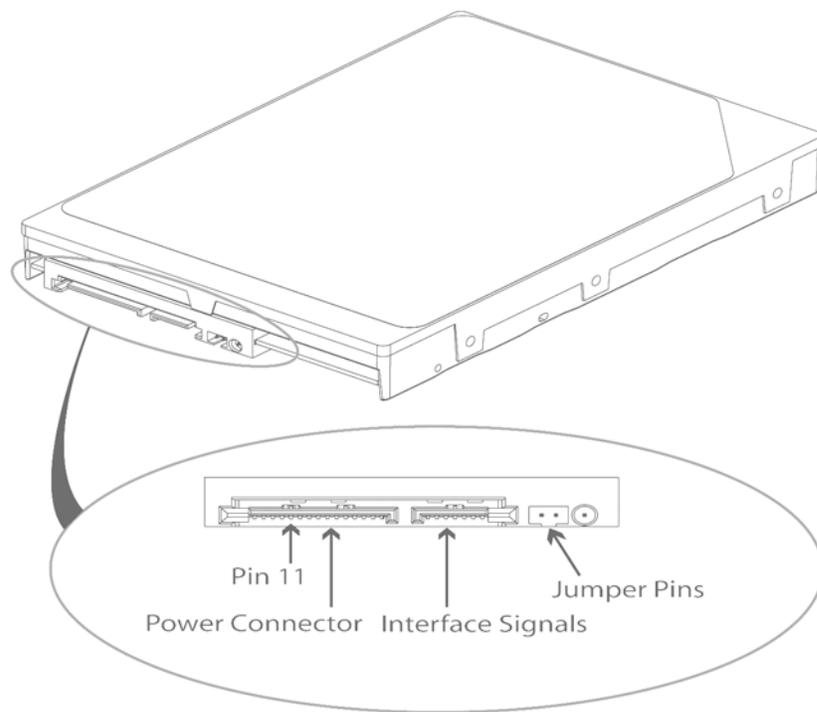
**Figure 4-4** DiamondMax 8S 40GB SATA Power/Interface Connector
