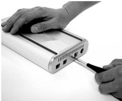
10. Secure the Back Panel with the 5mm diameter screw
