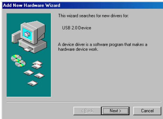
Power on the USB2.0 Enclosure and plug the USB cable into your USB2.0 port. The “Add New Hardware Wizard” should automatically appear as shown above. Click “Next” when this window appears.
