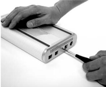
1. Do not connect AC Adapter to the enclosure. unscrew to loosen the Back Panel and remove the Back Panel from the Enclosure.
