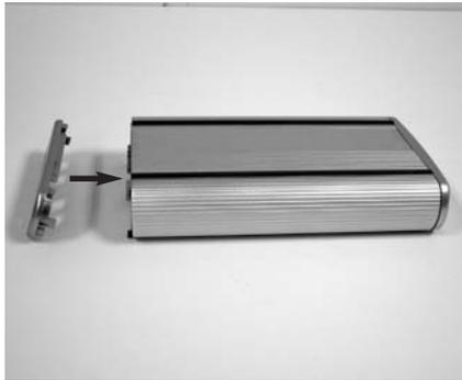
9. Install the Back Panel to the Enclosure..
