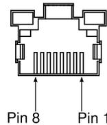
Figure 2.9. RJ45 Port Connector
