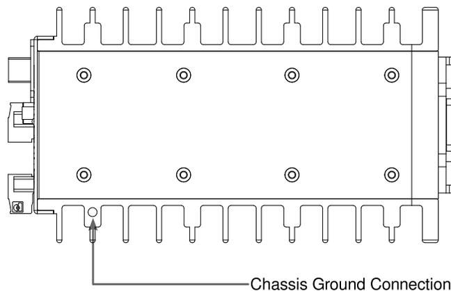
**Figure 2.6. RS900GP Chassis Ground Connection**
