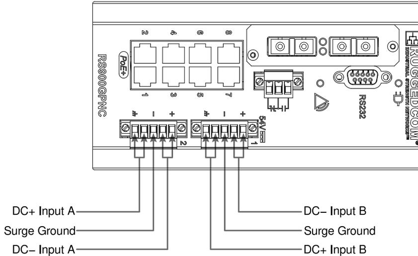
**Figure 2.5. DC Power Supply Wiring and Grounding**
