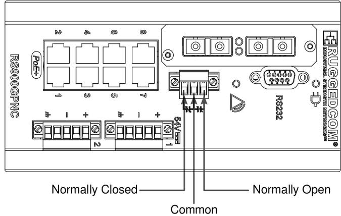
Figure 2.7. Failsafe Output Relay
