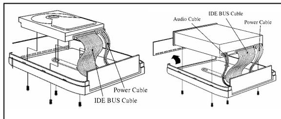
Connect the IDE and Power Cable to your HDD, CD-ROM, CDR(W) or DVD drive and the Audio Cable to your CD-ROM, CD-R(W) or DVD drive. If you use a CD-ROM, CD-RW or DVD drive, remove the front panel from the Housing. Mount the drive carefully on to the base and secure using the 4 screws supplied.
