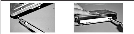
Mount the drive carefully to the 2 metal HDD mounting rails as shown above using the screws supplied.
