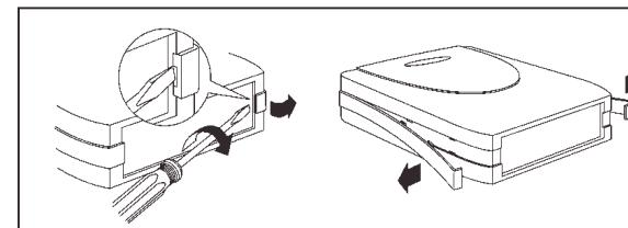
Carefully prise the two fixing rails **from the back** of the housing using a screwdriver. Strip the rails off carefully from back to front. Separate the top cover from the base.
