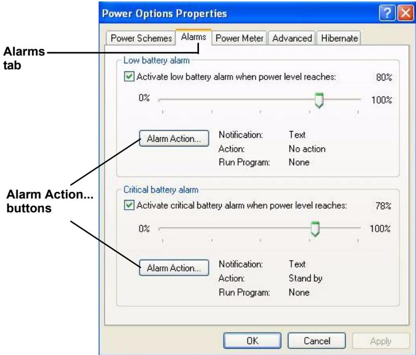
5. To enable automated shutdown for either alarm, select the associated **Alarm Action** button for the alarm you would like to configure.
