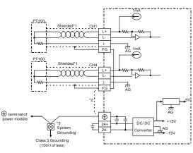
Note 1: Use only the wires that are packed with the temperature sensor (PT 100) for analog input and separate from other power line or any wire that may cause noise. Please use 3wire for PT
