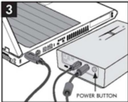
Connect the Hi-Speed USB 2.0 cable to your computer. Press the power button to switch on your SAFE Hard Drive.
