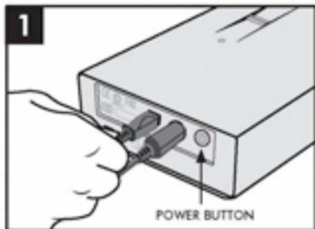
Connect the power supply and the Hi-Speed USB 2.0 cable. Press the power button to switch on the drive.
