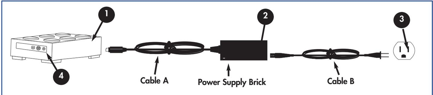
There are two cables that are supplied with the power supply: one cable (A) connects to a power outlet, such as a wall outlet or a surge protector; and the other cable (B) connects to the LaCie drive.
