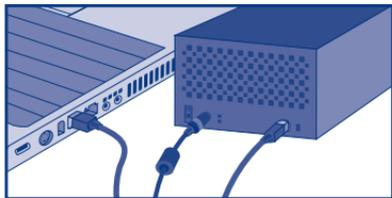
3. Turn on the hard disk MAX by moving the power switch on the back to the ON position.
