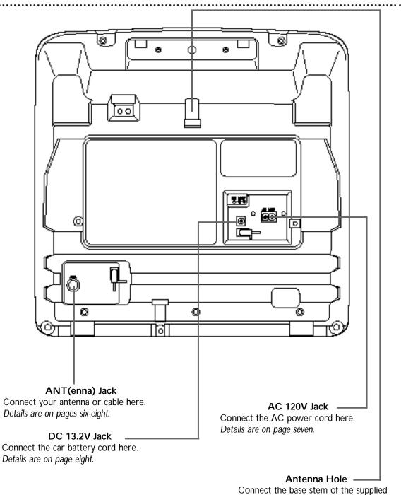
Connect the base stem of the supplied rod antenna here. *Details are on pages seven-eight.*
