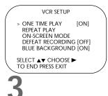
Press the PLAY/▲ button or the STOP/▼ button to select BLUE BACKGROUND. Then, press the F.FWD/▶ button repeatedly so that OFF (or ON) appears beside BLUE BACK-GROUND.
