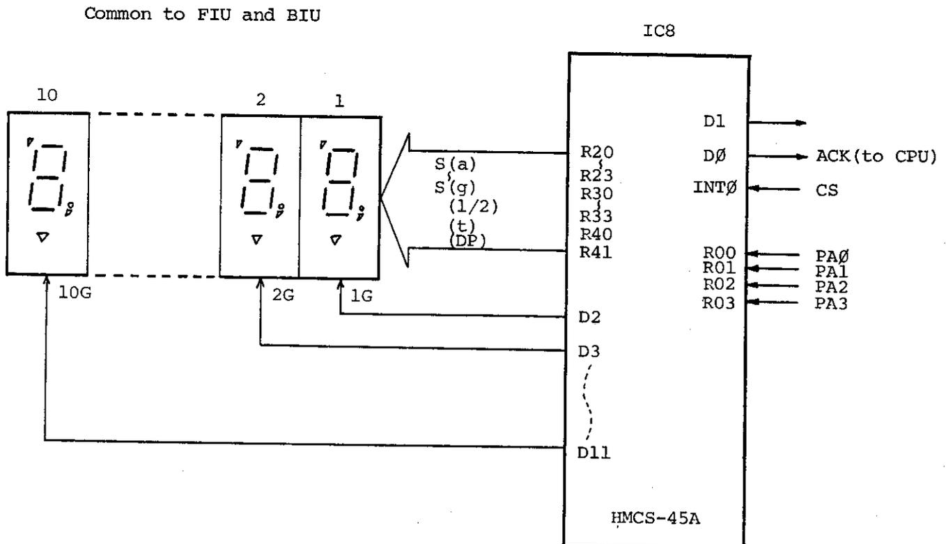
Fig. 6.1 Display Circuit Block Diagram
