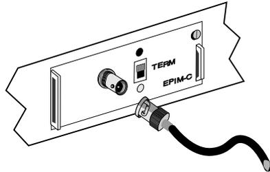
Attach thin-net segment directly to BNC connector when internal termination switch is set to on (●).
