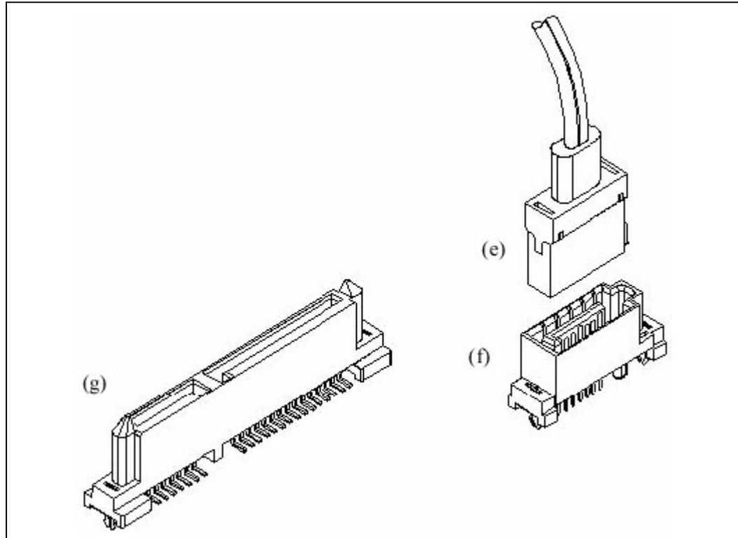
The signal cable receptacle connector on the other end of the cable is inserted into a host signal plug connector, shown as (f) in [Figure 22](#). The signal cable wire consists of two twinax sections in a common outer sheath.
