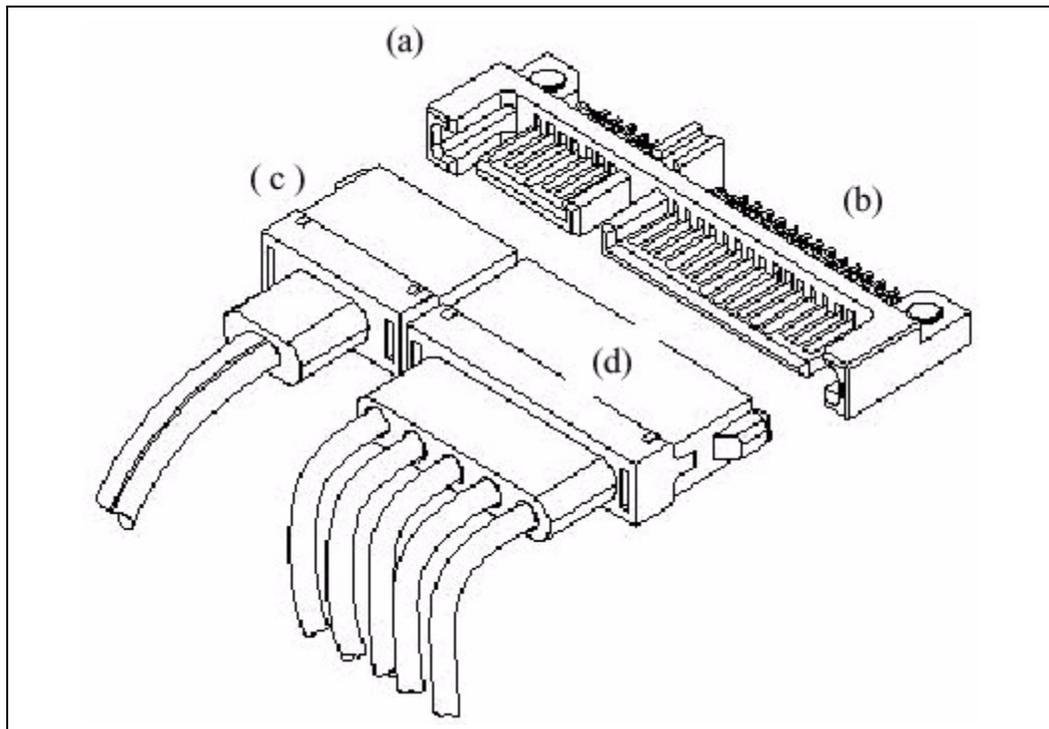
**Figure 22. Serial ATA Host Connectors**
