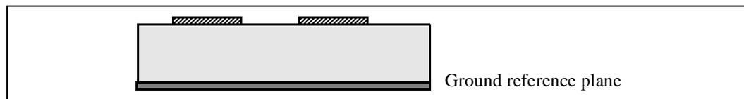
To calculate the coupled impedance requires a  $2 \times 2$  matrix. The diagonal values in the matrix represent the impedance of the traces to ground and the off-diagonal values provide a measure of how tightly the traces are coupled. The differential impedance is the value of the line-to-line resistor terminator that optimally terminates pure differential signals. The two by two matrix is shown below as:
