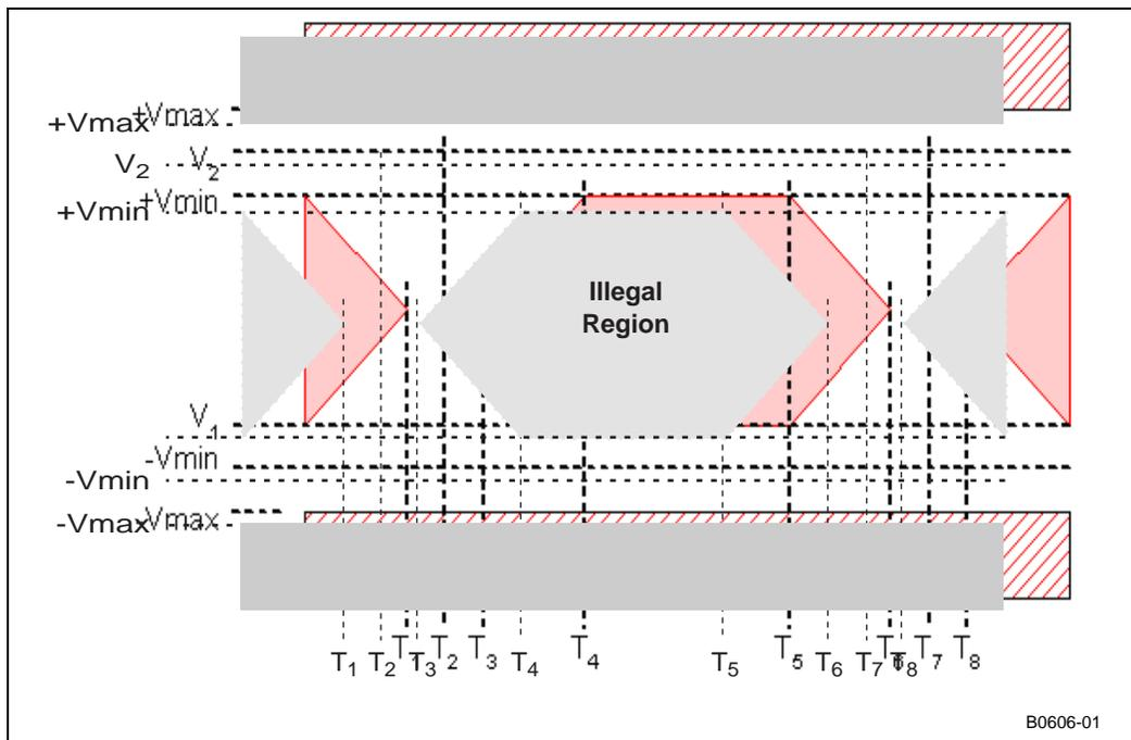
Several of oscilloscopes provide eye pattern masking options to allow the user to set up a mask for serial data streams such as Serial ATA. Automating this measurement through oscilloscope eye mask setup takes a the qualitative guess work out of eye pattern analysis.
