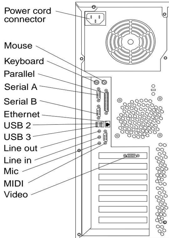
**Note:** If the server is a SCSI model, the SCSI adapter will be located in PCI slot 1; the external connector will appear in the slot below the video connector. See “System and PCI extender board options connectors” on page 35 for the location of the PCI slots.
