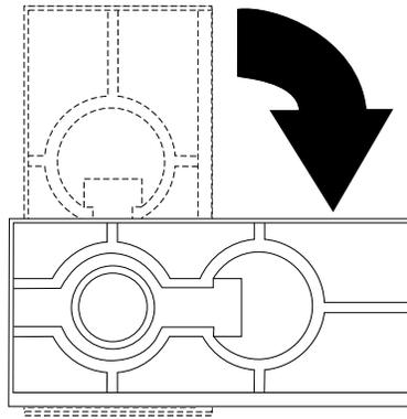
When you are finished installing options and have installed the side cover, turn the two front stabilizing feet a quarter turn out from the server and set it carefully back on its feet.
