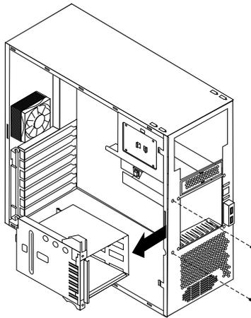
To remove the hard disk drive cage, do the following:
