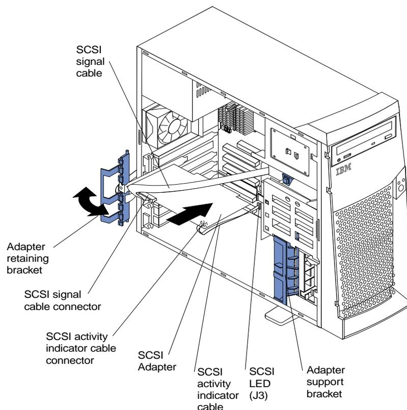
2. Connect the SCSI signal cable to the adapter and one or more of the signal cable connectors to the rear of the SCSI devices.
