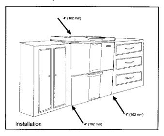
NOTE: The exterior walls of the freezer may become quite warm as the compressor works to transfer heat from the inside. Temperatures as much as 30°F warmer than room temperature can be expected. For this reason it is particularly important in hotter climates to allow enough space for air circulation around your freezer.
