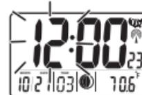
\*Press **MODE** again : the minute digits will flash and minute can be set by pressing **UP** [+] or **DOWN** [—] key.
