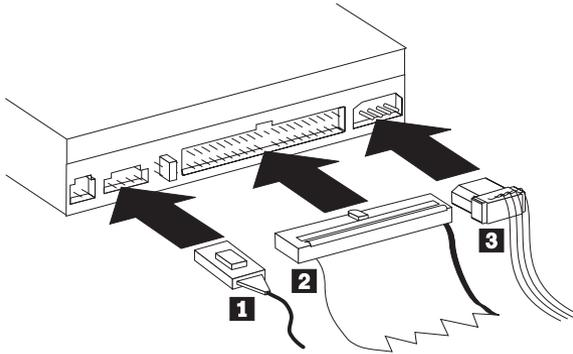
1. If you want to connect the CD-RW drive to your sound adapter or to the sound function on your system board, locate the included audio cables and determine which cable best fits the CD audio-in port on your sound adapter. Connect one end of the selected audio cable to the CD-RW drive audio-out connector **1**, and the other end of the cable to your sound adapter CD audio-in port. Save the other cable in case you use a different sound adapter in the future.
