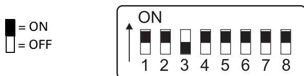
Figure 1.3 Configuration switches (shown in default positions)
