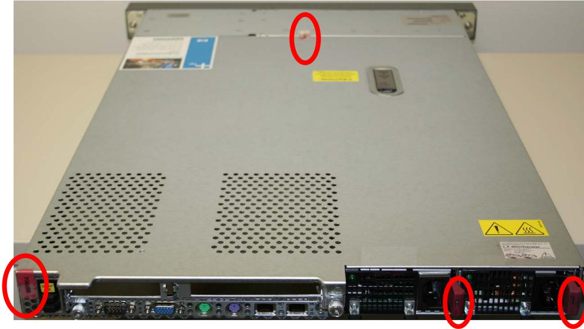
**Figure 8 – Tamper-Evidence Labels**
