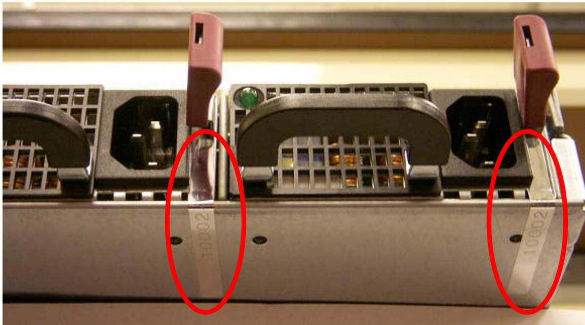
**Figure 9 – Tamper-Evidence Labels over Power Supplies**
