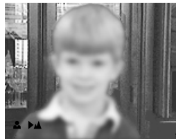
Focus indicators tell whether the camcorder is focusing on the foreground or background
