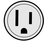
Two-Pole, 3-wire Grounding Receptacle 15 Amps. 125V.
