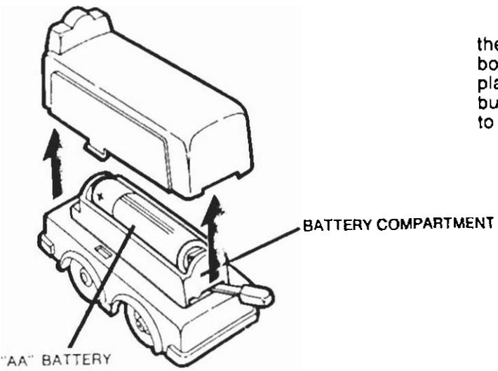
**4** To make the bus run on the track, flip down the posts on the bottom of the bus. For free-wheeling floor-play, flip up the posts on the bottom of the bus. To start the bus, move the start switch to the "ON" position.
