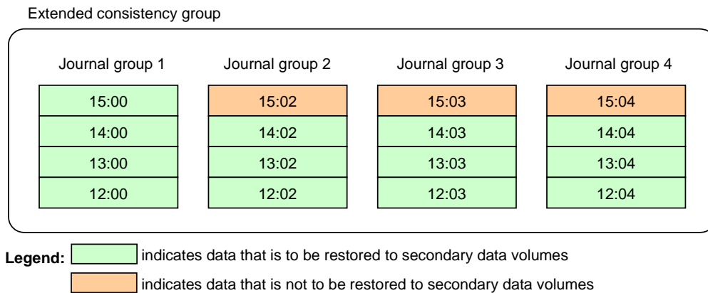
Figure 2-4 Time Stamps of Data that Have Not Been Restored to Secondary Data Volumes
