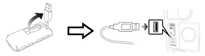
Your USB Hub comes with an additional USB Power Cable. The use of this USB Power Cable is recommended for additional power if multiple devices or high power consumption devices such as Micro Drives or Bus Powered USB devices are connected to your USB Hub. To connect your USB Hub with the enclosed USB Power Cable, please refer to the diagram shown below:
