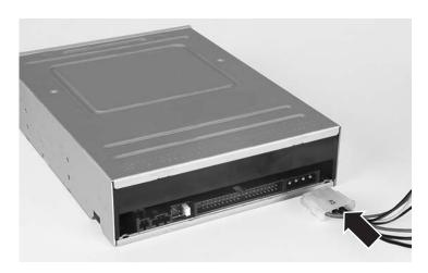
If you do not have enough power connectors, disconnect a power cable from one of your drives and place the Y-adapter power cable that came with the new drive on the end of the existing power cable to make two power connectors.
