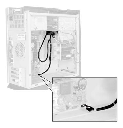
**6** Disconnect the power cable from the back of the drive. Make sure that you pull the connector, not the cable. Move the connector slightly side-to-side, if necessary, to disconnect the cable.
