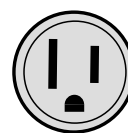
3-pronged Grounding Receptacle 15 Amps. 125V.
