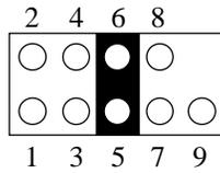
CSEL connected to the interface cable selection can be done by the special interface cable.
