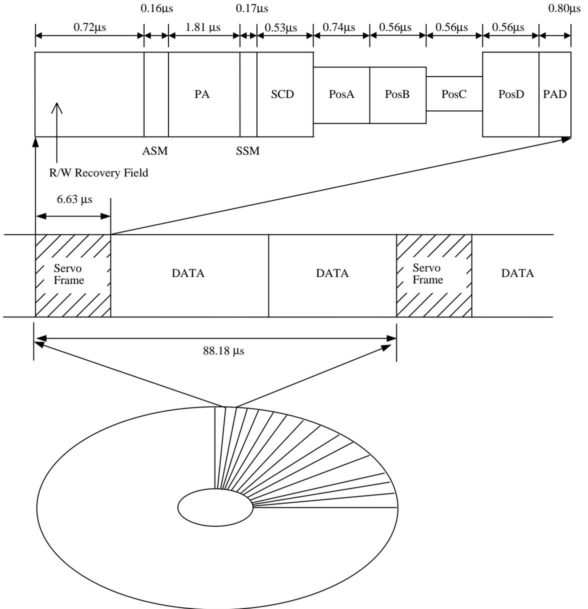
Figure 4.6 126 Servo frames in each track
