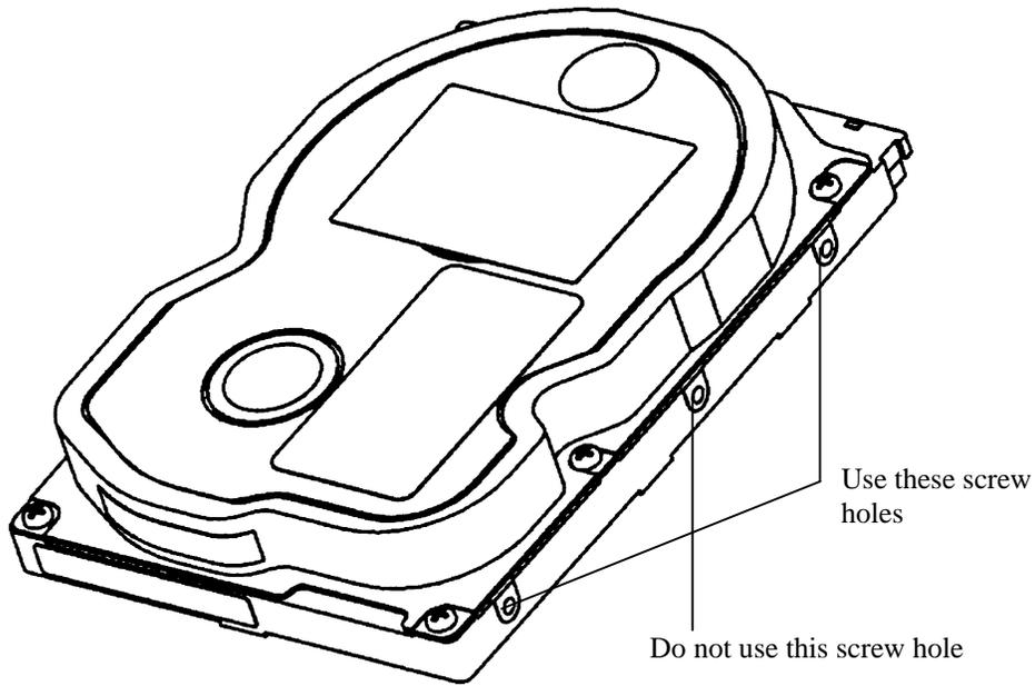
**Figure 3.4** Limitation of side-mounting
