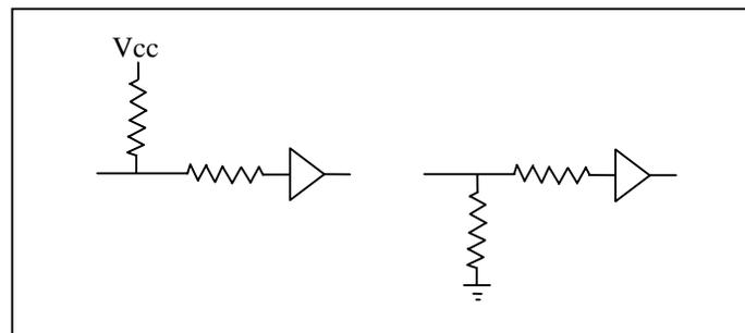
**Figure 5.7 Ultra DMA termination with pull-up or pull-down**
