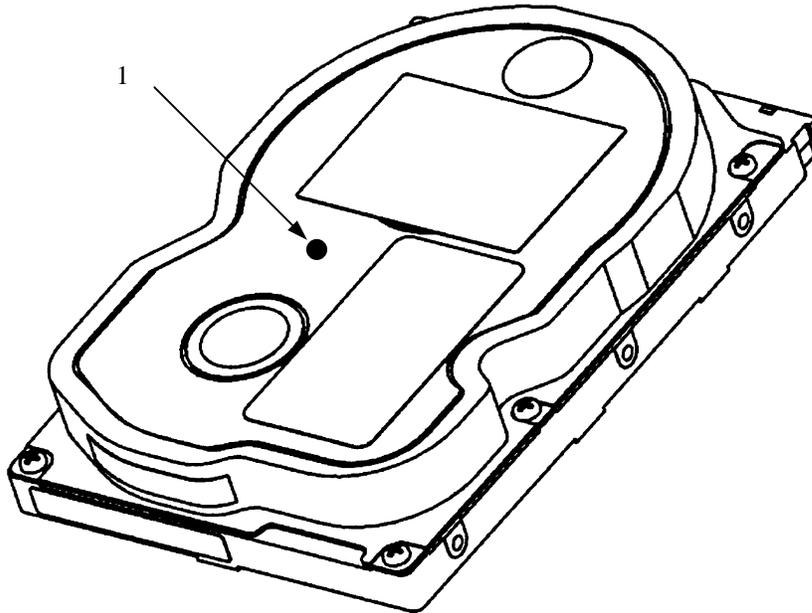
**Figure 3.6** Surface temperature measurement points
