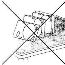
Do not place HDD vertically to avoid falling down.
