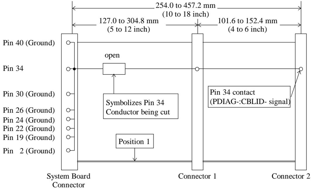
**Figure 3.11 Cable configuration**
