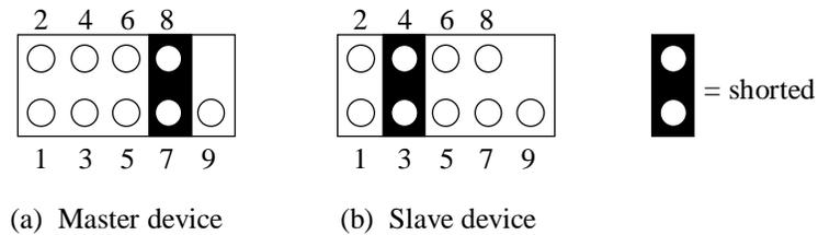
Figure 3.16 Jumper setting of master or slave device
