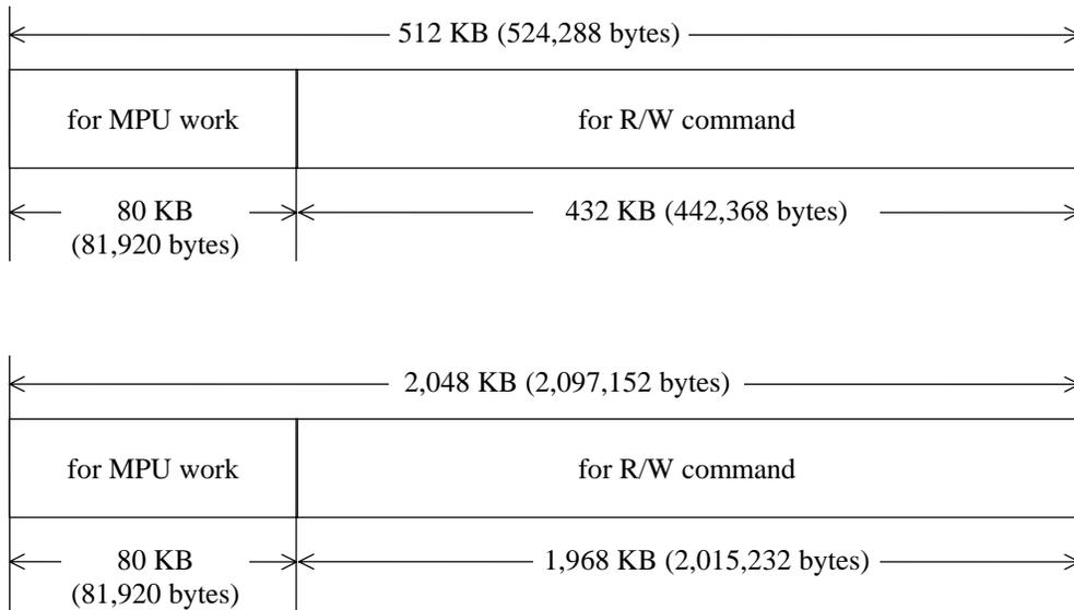
**Figure 6.9 Data buffer configuration**
