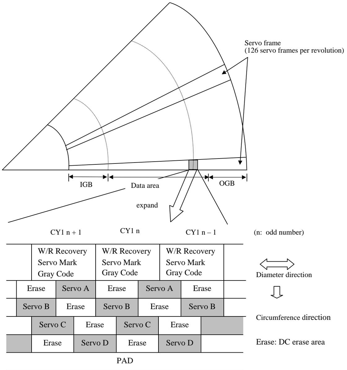
**Figure 4.5 Physical sector servo configuration on disk surface**
