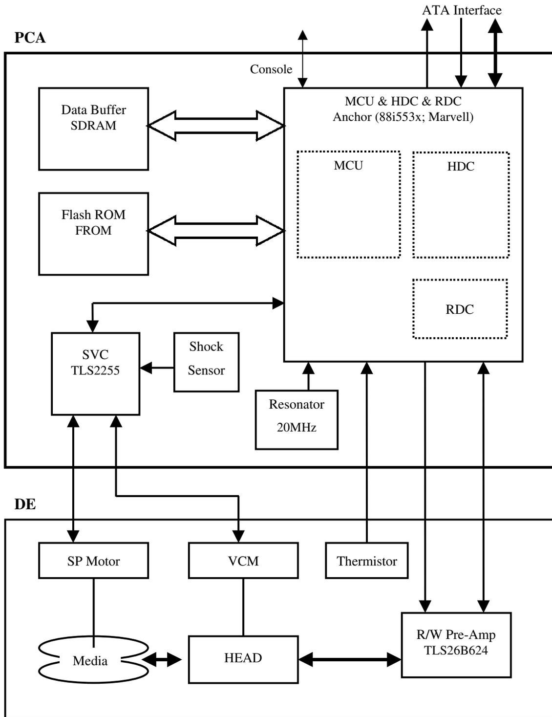
Figure 4.2 Circuit Configuration
