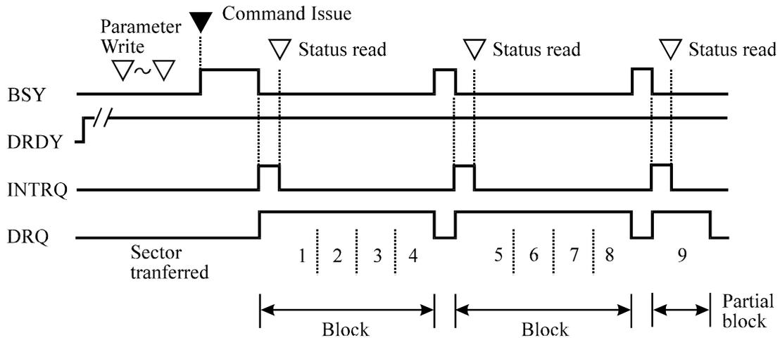
**Figure 5.2 Execution example of READ MULTIPLE command**
