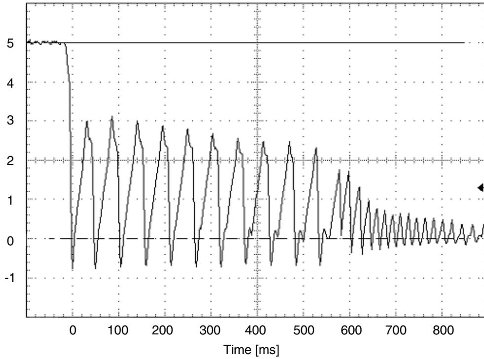
**Figure 1.1 Negative voltage at +5 V when power is turned off**
