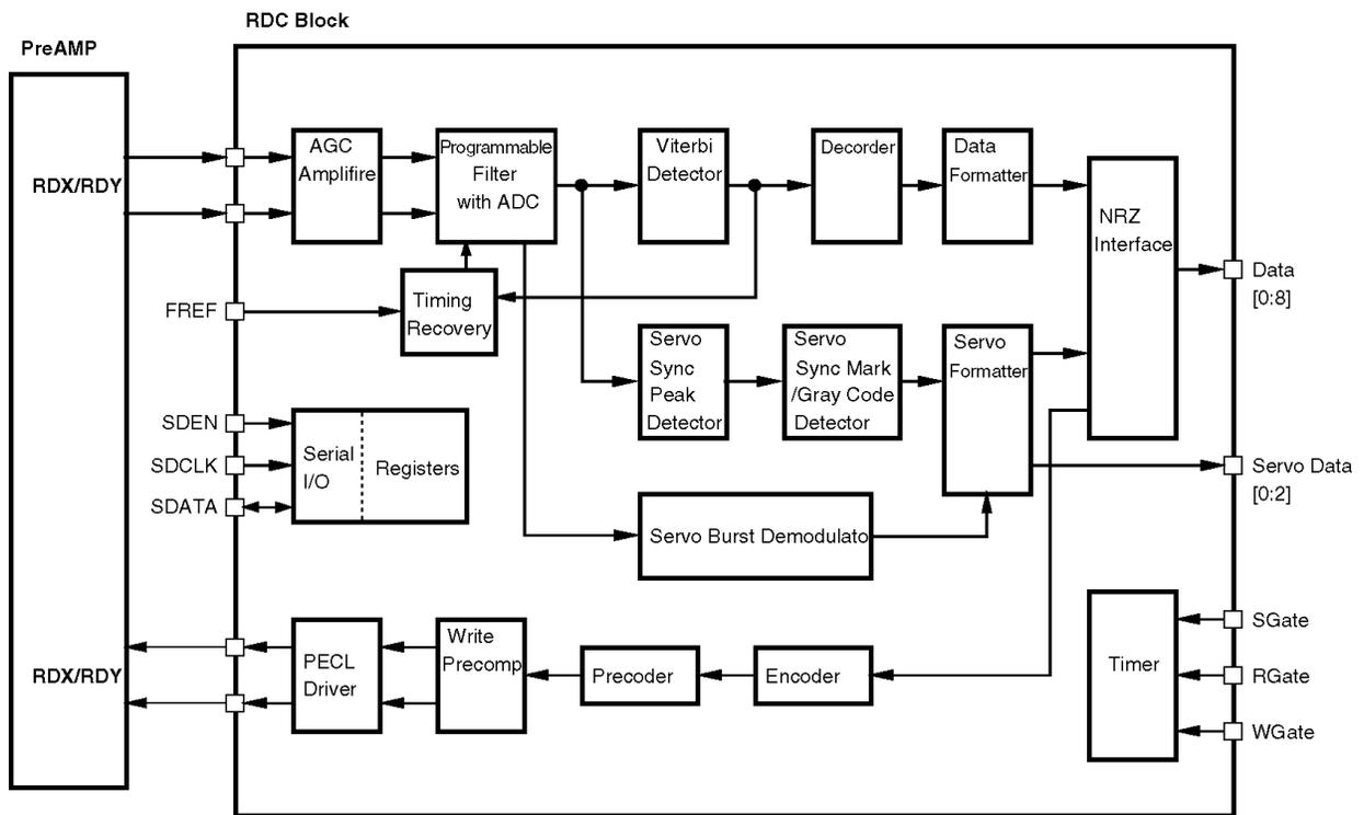
Figure 4.4 Read/write circuit block diagram
