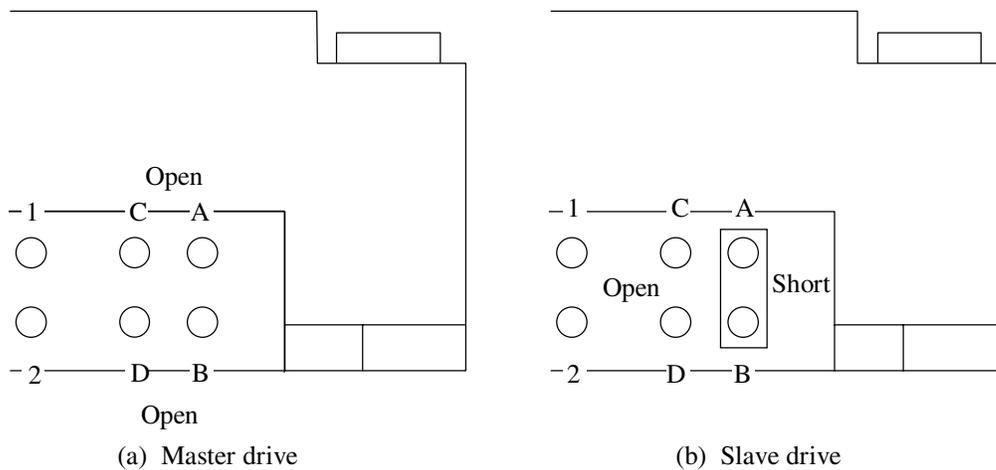
**Figure 3.13 Jumper setting of master or slave drive**
