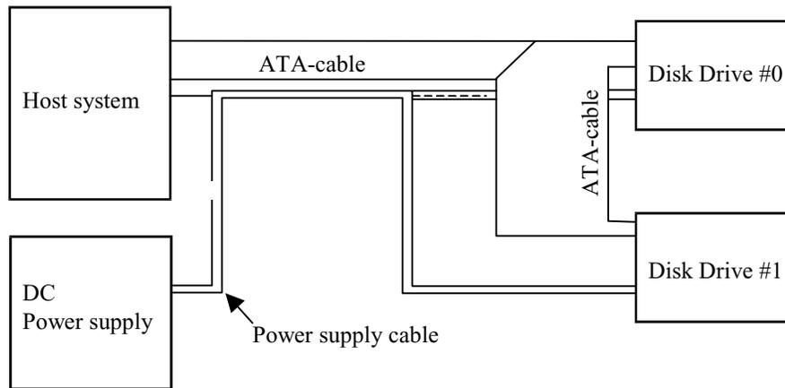
**Figure 3.9 Cable connections**
