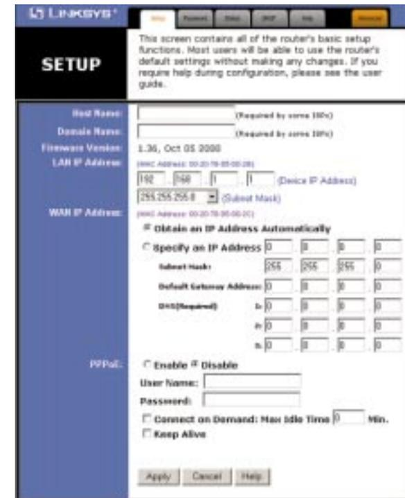
The Basic Setup screen is the first screen you will see when you access the Utility. If you have already installed and setup the Router, you have already seen this screen and have already properly configured all of the screen's values.
