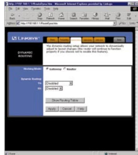
With Dynamic Routing you can automatically adjust to physical changes in the network's layout. The HomeLink Phoneline Router, using the RIP protocol, determines the network packets' route based on the fewest number of hops between the source and the destination. The RIP protocol regularly broadcasts routing information to other routers on the network.
