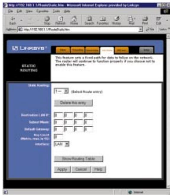
If your HomeLink Phoneline Router is connected to more than one network, it may be necessary to set up a static route between them. A static route is a pre-determined pathway that network information must travel to reach a specific host or network. Click the **Show Routing Table** button to view the current static routing configuration.
