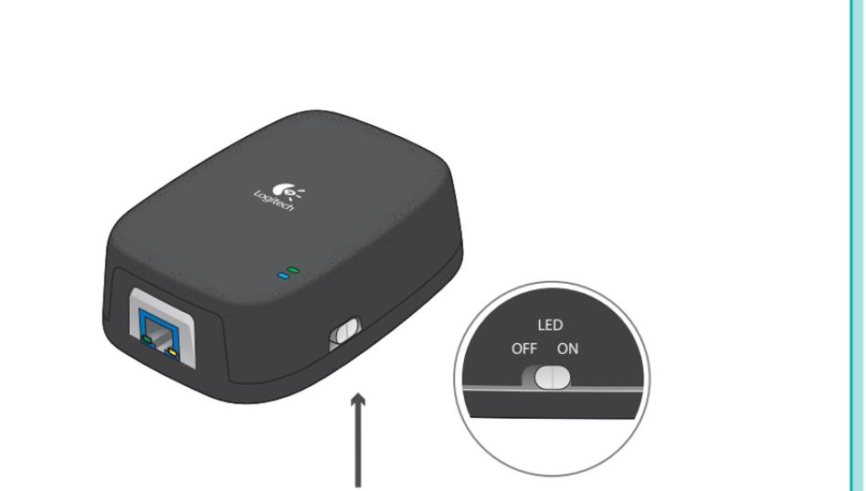
Use the switch on the side of the network adapter to disable the diagnostic and status LEDs.
