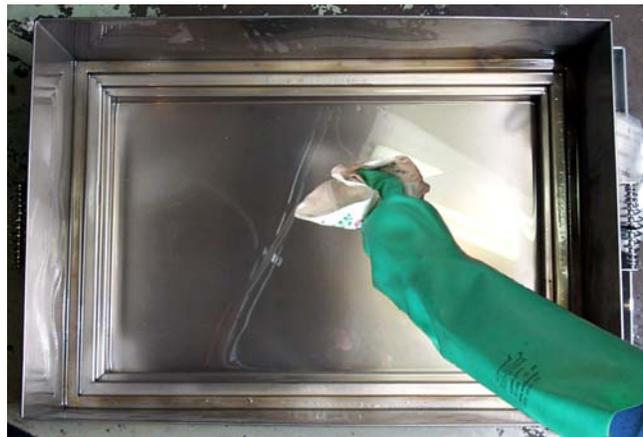
Ensure filter pan and all components are clean and dry before installing filter leaf assembly and crumb tray.
