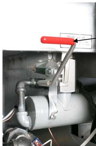
YSCFC24 drain valve and handle. Move the red drain handle down to open the valve, draining the frypot into the filter pan.
