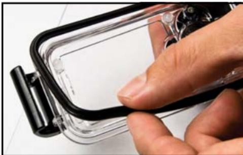
3. To install a new or clean seal, start at any corner, push the seal into the corner and run your finger along the seal to ensure it is seated completely on all four sides and corners.
