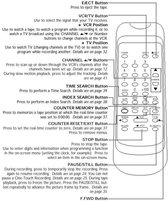
When tape playback is stopped, press to fast forward the tape at high speed. During tape playback, press to fast forward the tape while the picture stays on the screen. Details are on page 35. Press to change the setting of an item in the VCR menu or press to proceed to the next menu.
