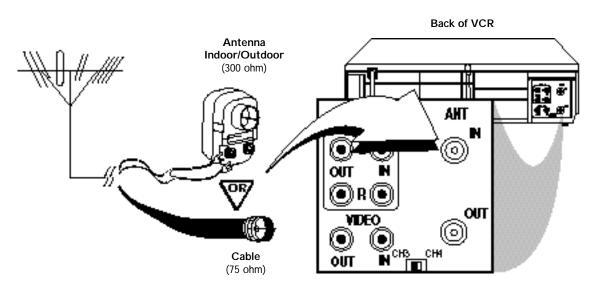
Connect the RF coaxial cable (supplied) to the OUT Jack on the back of the VCR and to the ANTENNA IN Jack on the TV. (You may use either a snap-on type (supplied) or screw-on type of coaxial cable, whichever you prefer.)
