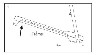
Hold the treadmill firmly with your right hand as shown. Pull the latch knob to the left and hold it. Raise the frame until the latch plate is past the latch pin. Then, slowly release the latch knob; make sure that the frame is held securely by the latch pin.
