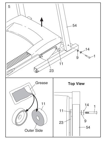
See the left inset drawing in step 5. Identify the outer side of the remaining Frame Spacer (11).
