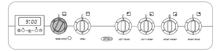
To operate the oven turn the oven temperature control clockwise to the required setting.
