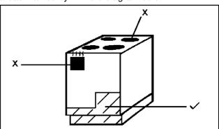
To move the cooker, open the oven door and lift the cooker by holding inside the top of the compartment.
