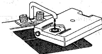
Grasp the water bottle handle, and lower into the cabinet. The "E-Z-Fill Side-Cap" must be facing the center of the cabinet. When positioned properly, the plunger will open and water will flow into the cabinet. The water level will automatically remain at approximately 1" until the bottle is empty. The unit is now ready for operation.
