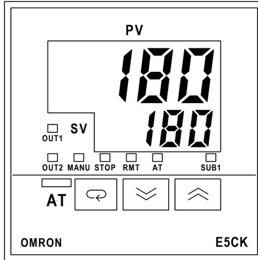
**Note:** The only functional buttons on this controller are the up and down keys.
