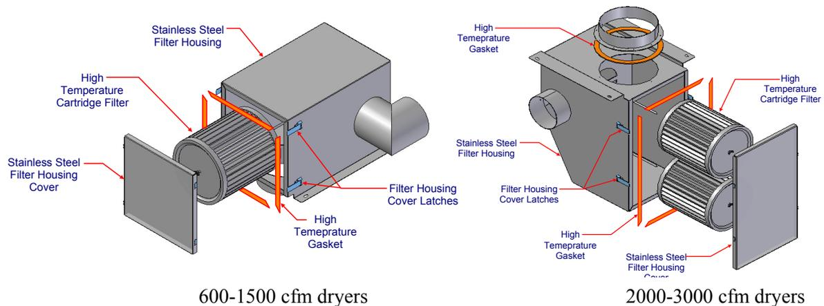
Use the following procedure to clean or replace the filter cartridges:
