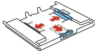
5. Set the front edge guide to the position for the paper size you are using.
