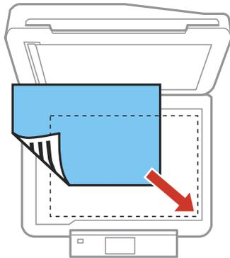
**Note:** You can place multiple originals on the scanner glass. Just make sure they are at least 0.20 inch (5 mm) away from each other and from the edge of the scanner glass.
