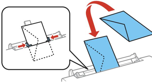
5. Push the paper or envelope down until it meets resistance. About 2 inches (5 cm) of the paper should be fed inside the printer as shown.
