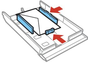
**Note:** Make sure the envelopes are under the tabs on the edge guides.
