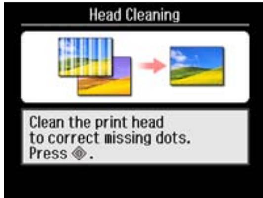
7. Press the  $\diamond$  start button to clean the print head. You see a message on the LCD screen during the cleaning cycle.
