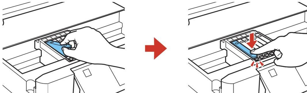
9. Once you replace all the cartridges that need replacing, close the scanner unit.
