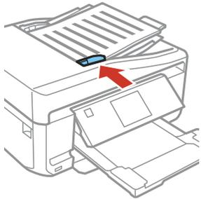
**Note:** If you're using the **Letter, 2-up Copy**, or **A4, 2-up Copy** layout, make sure the originals are loaded as shown.
