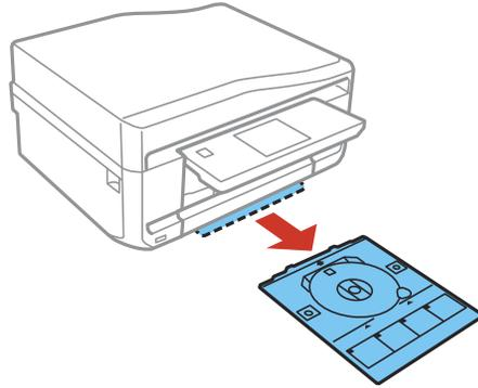
9. Place a CD or DVD on the CD/DVD tray with the printable side faceup, and insert the tray into the slot above the output tray.
