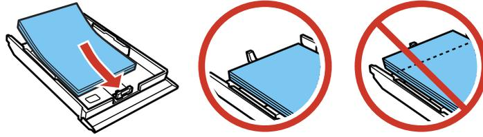
**Note:** Make sure the paper is loaded against the edge guide and not sticking out from the end of the cassette.
