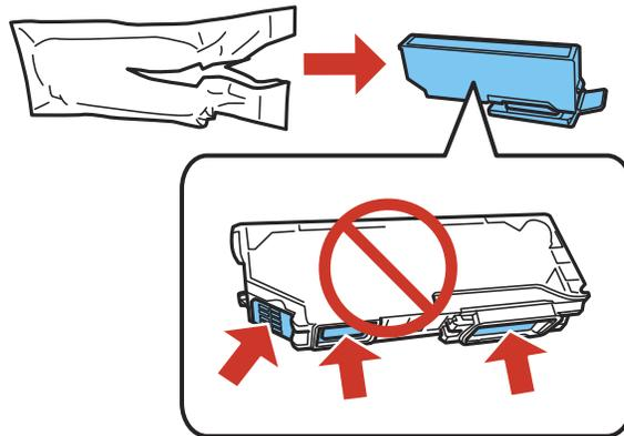
**Caution:** Do not shake the cartridges after opening the packages, or ink may leak. Do not touch the areas shown above. Doing so may prevent normal operation and printing.
