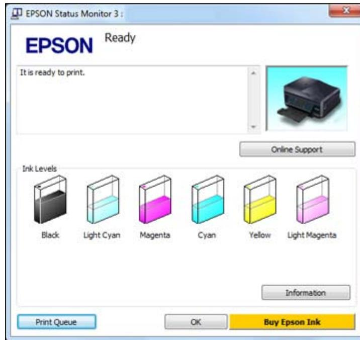
2. Replace or reinstall any ink cartridge indicated on the screen.
