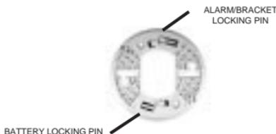
2. Insert the pin into the hole for the feature you are activating. Refer to the diagram below for correct placement.
