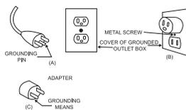
This product is for use on 120 volts. The cord has a plug (A) as shown. An adapter (C) (not included) is available for connecting three-blade grounding-type plugs to two-slot receptacles (B). The green grounding lug extending from the adapter must be connected to a permanent ground such as a properly grounded outlet box. The adapter should not be used if a three-slot grounded receptacle is available.
