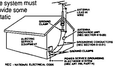
regarding proper grounding of the mast and supporting structure, grounding of the lead-in wire to an antenna discharge unit, size of grounding conductors, location of antenna discharge unit, connection to grounding electrodes, and requirements for the grounding electrode.
