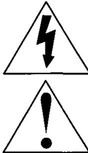
This symbol warns the user that uninsulated voltage within the unit may have sufficient magnitude to cause electric shock.
